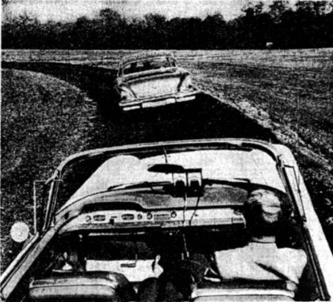
In test at R. C. A. Laboratories, Princeton, N. J., driverless car, foreground, is guided by impulses from wires buried in road. It will remain safe distance behind car ahead.
